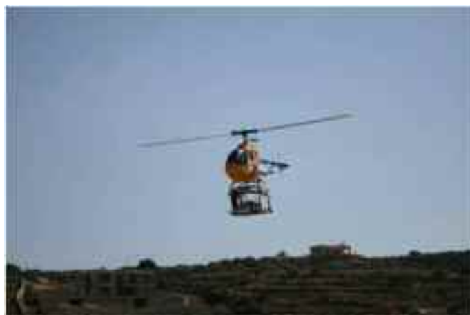
Mini-Helicopter for Radioactive Material Detection at NMIOTC Experiments
