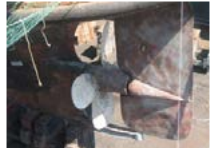
Fig. 7: The predecessor of Promas on a 1943-built tugboat
