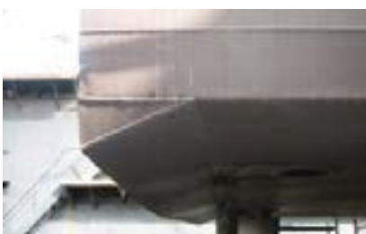
Fig. 5: A stern wedge retrofit on a Hellenic Navy FPBM
