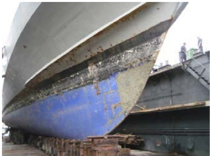
Fig. 8: FR coatings on a Hellenic Navy fast patrol boat after 12 years
