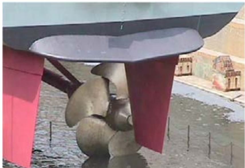
Fig. 4: Stern flap installed on a DDG-51
