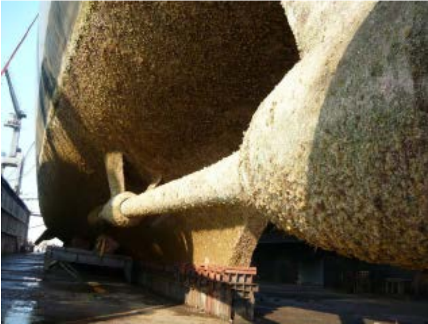
Fig. 3: Hard fouling on an S-type frigate of the Hellenic Navy
