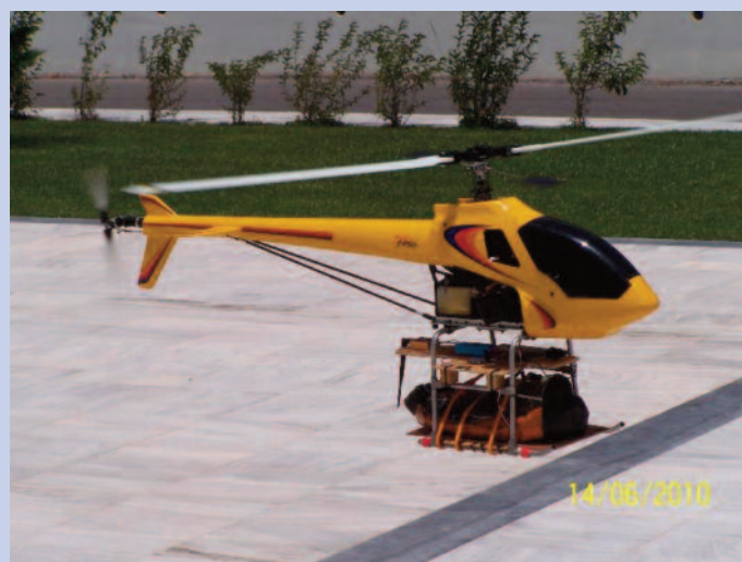
Fig 1. UAV mini helo with the LLNL Sensor onboard during test flights in NMIOTC’s premises
