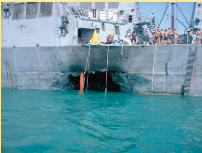
Fig. 2: USS Cole in Port of Aden attacked from a small inflatable boat in a terrorist/ pirate act [6,7]. WIEDs were used in order to provoke this criminal result
