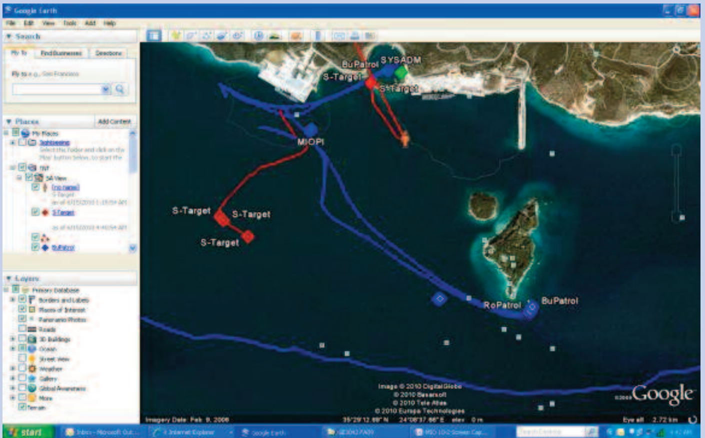
Figure 8. NMIOTC Romanian and Hellenic boats comprise mesh networking relays to assist Bulgarian sensor boat continuing non-LOS stand-off detection behind the island.
