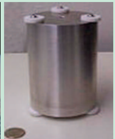
Tubesat Pico satellite pictures (courtesy Interorbital Company). This Pico satellite is going to be used from NPS in order to send and receive messages regarding WMD in Maritime Interdiction Operations. The amazing fact though is that as it can be seen from the right picture this pico satellite is weighting only 0.75 kgr and it has the dimensions of a typical small glass of water. With this technology the cost of using pico satellites in WMD MIO operations is minimal for every possible user.
