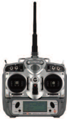
Fig 2: (a) Heli Control Unit
