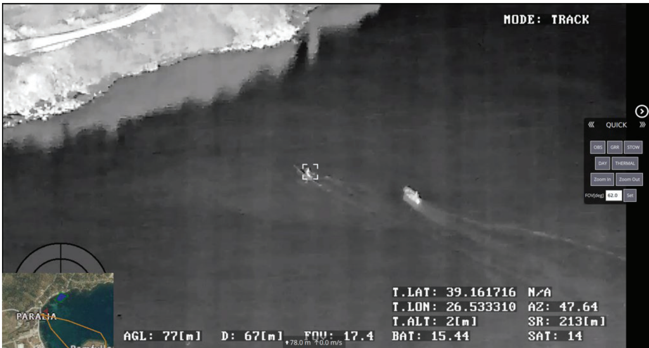
Figure 2: User interface of the ARSx2 system. The thermal channel is active while a subject is 'locked' and tracked during field tests. Information about the subject are calculated continuously.
